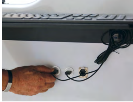
Connect the mouse and keyboard to the USB jacks on the right-side front panel.
