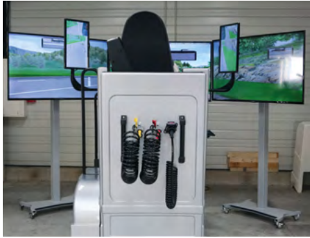
The left and right screens correspond respectively to the left and right sight of the user
